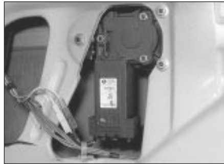
23.3 Electric window regulator unit and wiring connections
