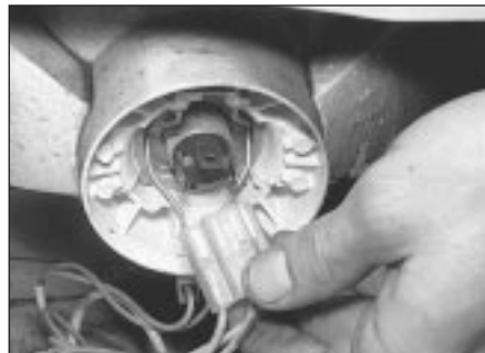
3.2a Disconnect the wiring connector . . .
