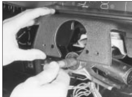
9.13a Removing the steering column upper shroud
