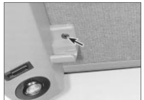
4.4a Map reading light switch and roof console retaining screw (arrowed)
