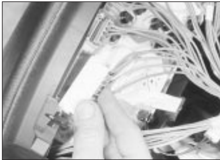
7.17a Instrument panel wiring connectors
