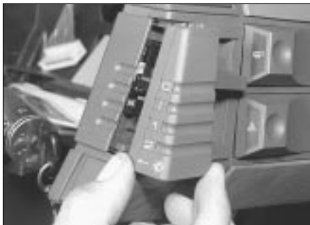
9.3 Removing a central panel
