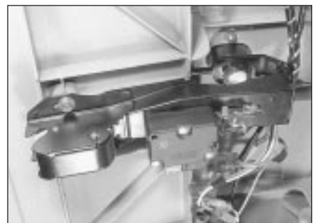
25.10 Tailgate central locking solenoid and lock unit
