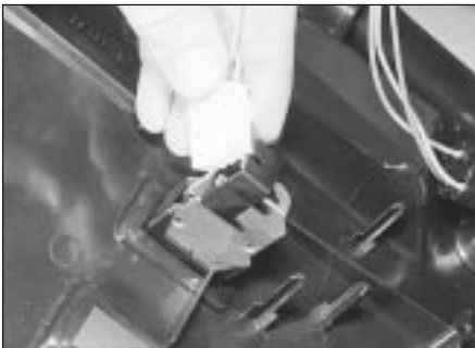
9.12 Detaching the wiring plug from the instrument lighting rheostat
