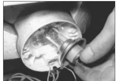
3.2b . . . and remove the headlight bulb
