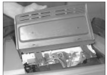
7.2 Instrument panel inspection cover removal
