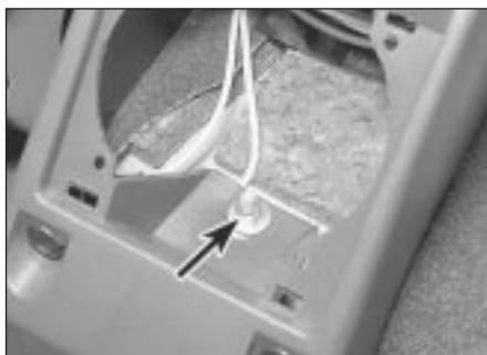
13.2 Handbrake console retaining nut (arrowed)
