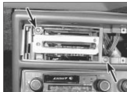
28.4 Remove the panel screws indicated
