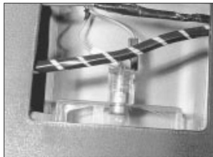
3.25 Number plate light unit shown with access cover removed from trim panel (Hatchback)
