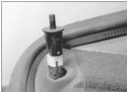
10.5 Boot light switch unit removal
