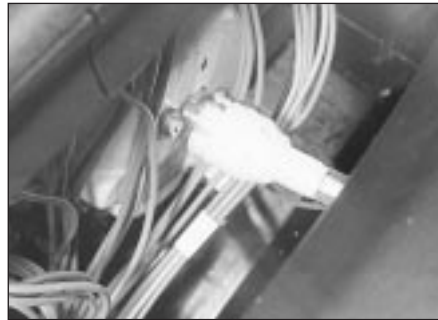
7.17b Speedometer cable connector
