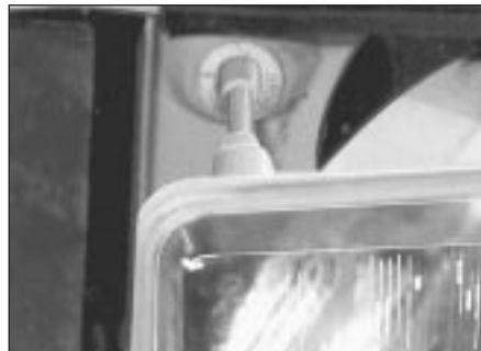
3.6 Headlamp ball and socket mounting
