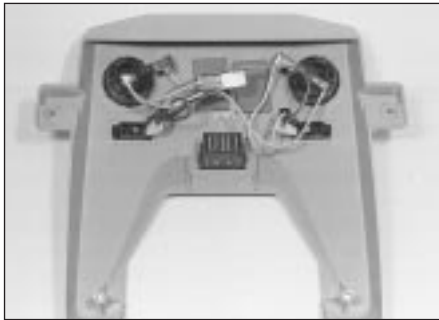
4.4b Map reading light/ sunroof console removed
