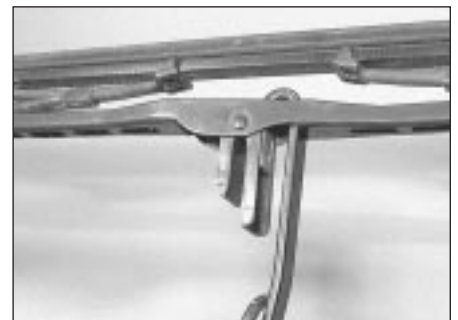
17.2 Wiper blade removal from arm
