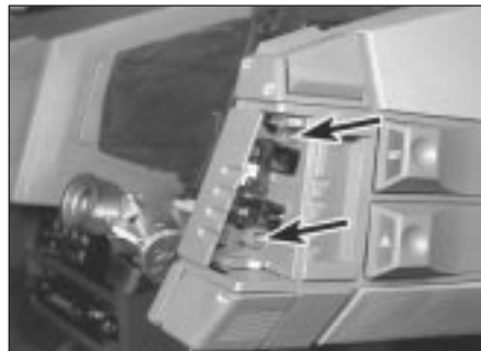
9.4a Remove the two retaining screws (arrowed) . . .
