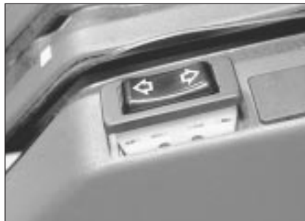
11.2 Electric window operating switch removal
