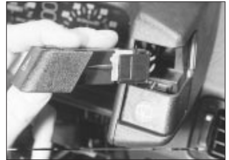
8.2 Removing a facia switch
