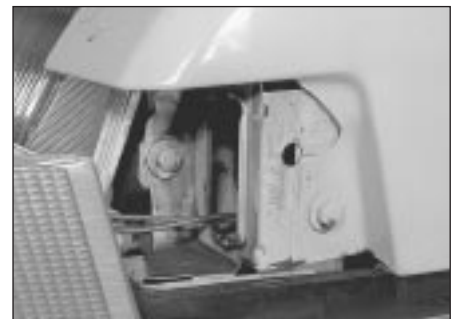
3.13 Withdraw the front indicator unit . . .
