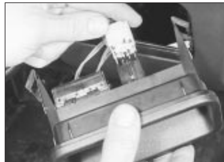
12.3a Disconnecting the wiring from the front foglight switch
