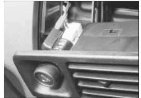
14.8 Withdrawing the grille panel
