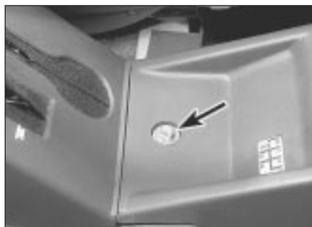
13.3 Console retaining bolt (arrowed)
