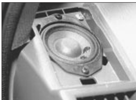
29.2 Facia-mounted speaker (upper) shown with grille panel removed
