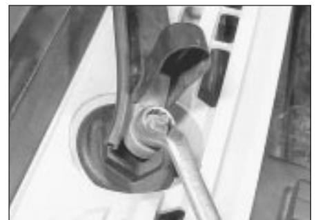
18.3 . . . and unscrew the wiper arm retaining nut
