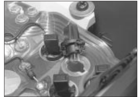
7.7 Bulb holder removal from the instrument panel
