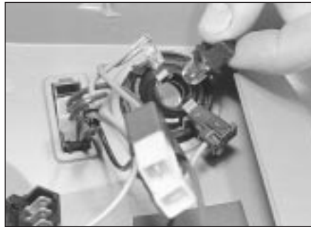
4.4c Removing the map reading light bulb
