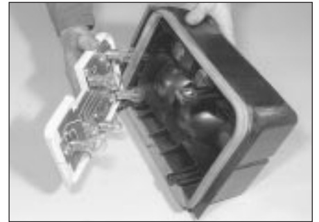
3.19 Removing the bulb holder from the rear lens unit (Hatchback)
