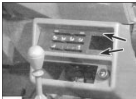
28.3 Ashtray holder/heater control plate retaining screws (arrowed)
