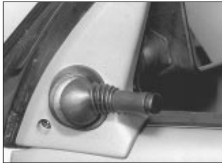
10.1 Door mirror adjuster knob and gaiter
