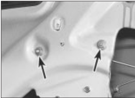
14.2 Door glass runner channel retaining nuts (arrowed)
