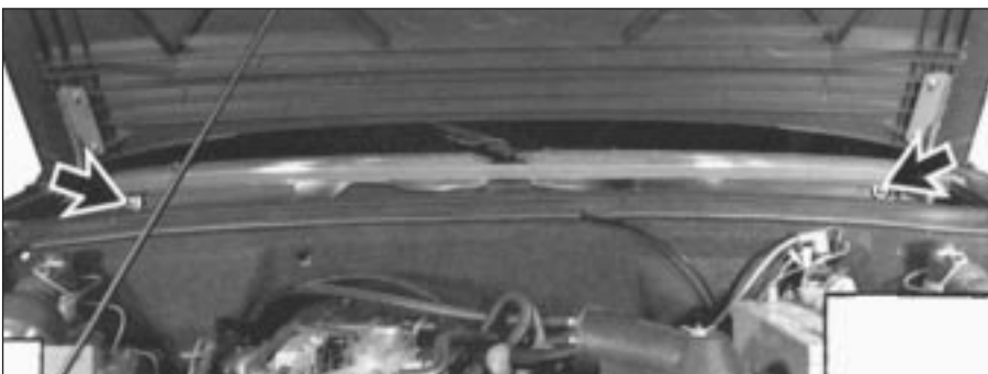
24.10 Undo the two retaining bolts (arrowed)
