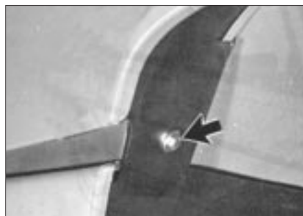
8.6 Remove single retaining bolt and washer (arrowed) from the front wing
