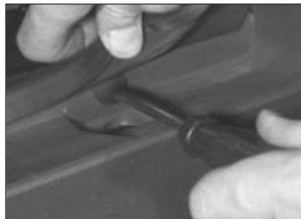
20.11b Unscrewing a rear bumper upper screw
