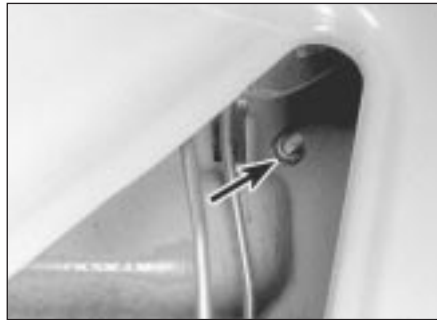
17.8 Door outer handle retaining nut (arrowed)
