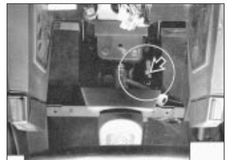
24.5 Detach the wiring connector (arrowed)
