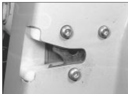
17.2 Door lock retaining screws and nylon grommet
