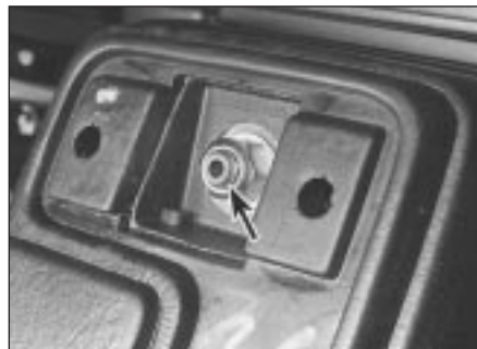
16.15b . . . to expose wheel retaining nut (arrowed)
