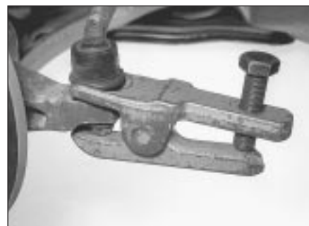
13.2b . . . and use a separator to detach the joint
