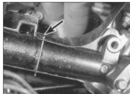
20.5b . . . and release retaining clip on underside (arrowed)
