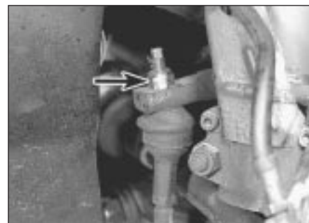
3.11 Anti-roll bar and connecting rod. Remove retaining nut (arrowed)
