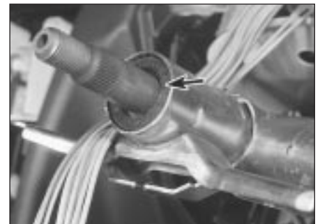
16.17 Upper steering column oil seal (arrowed)
