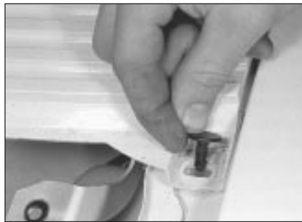
13.14 Removing an air inlet grille securing clip
