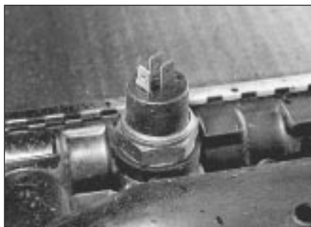
3.3 Temperature sensor unit location in radiator
