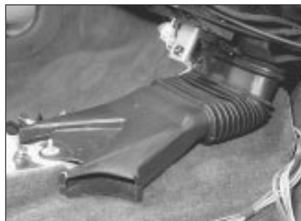
11.17 Rear passenger compartment heater nozzle
