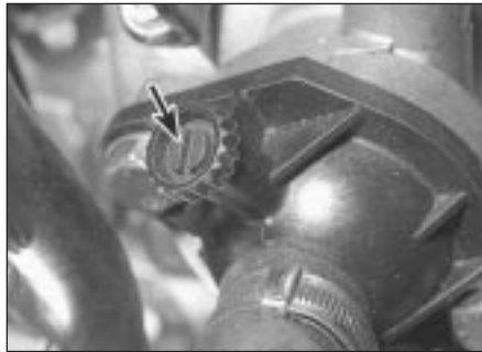
8.1c Thermostat housing bleed screw (arrowed) - BX 19 GTi 16v
