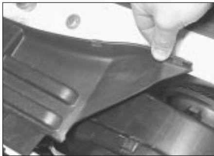
13.13 Removing plastic cover from heater blower motor
