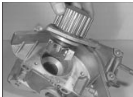
9.19a Removing coolant pump from housing
