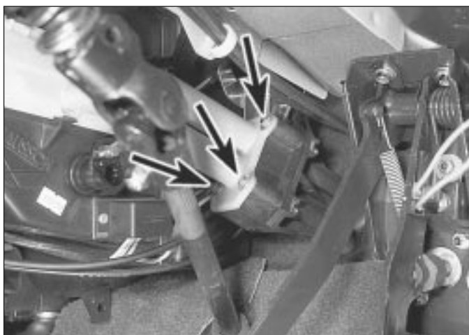
14.3 Heater tap (control) unit retaining screws (arrowed)
