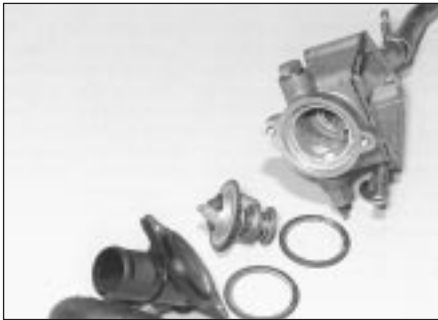
8.1b Thermostat housing dismantled - BX 19 GTi 16v
