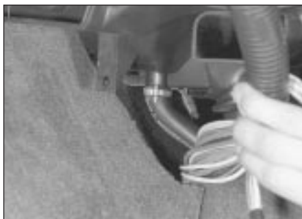
11.27 Heater coolant drain hose
