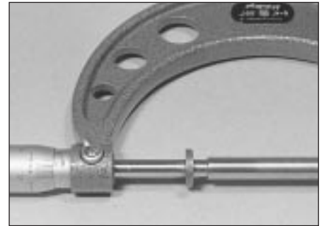
22.11b Measuring shim thickness with a micrometer
