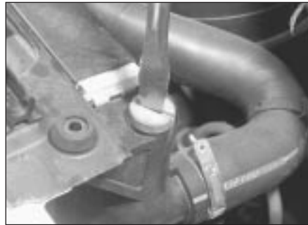
32.2b The radiator bleed screw - all models
