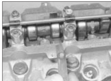
22.5b Measuring a valve clearance - 171 and 159 engines
