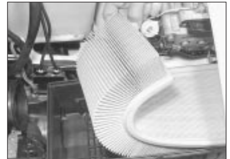
28.14 Lifting the air filter element from its housing - Motronic and Bosch systems
