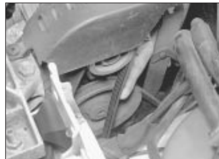
19.2 Checking alternator drivebelt tension
