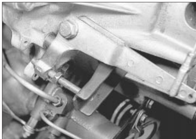
11.5 Clutch pushrod and release lever - BX 16
